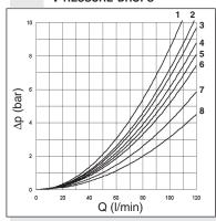
The diagram at the side shows the pressure drop curves for spools during normal usage. The fluid used is a mineral oil with a viscosity of 46 mm²/s at 40°C; the tests have been carried out at a fluid temperature of 40°C. For higher flow rates than those in the diagram, the losses will be those expressed by the following formula:
